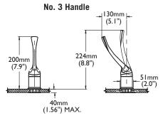
INLET FOR 3/8" OR 1/2" FLEXIBLE RISER OR 1/2-14 NPSM COUPLING NUT (NOT SUPPLIED)
